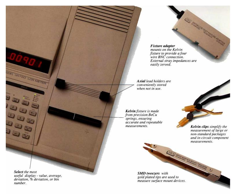
Both instruments feature a built-in Kelvin test fixture ensuring accurate measurements. Fixture compensation is performed quickly and easily from the front panel. Precision four wire measurements of resistance, inductance or capacitance, and Q, R or D completely characterize components.
